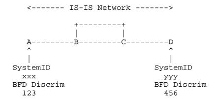
Figure 1: S-BFD for IS-IS Network
