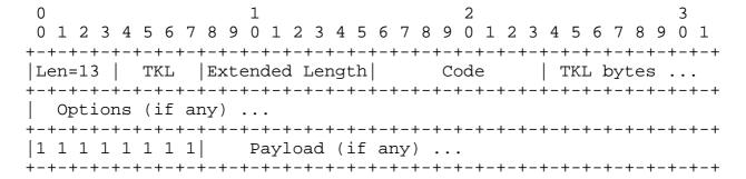
Figure 4: CoAP frame with 8-bit Extended Length field.
