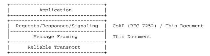
Figure 1: Layering of CoAP over Reliable Transports
