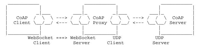
Figure 11: CoAP Client (WebSocket client) accesses CoAP Server (UDP server) via a CoAP proxy (WebSocket server/UDP client)
