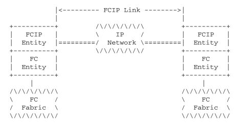
Fig. 3 Model for Two Connected FC/FCIP Entity Pairs
