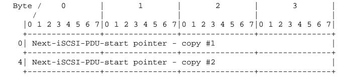
The Marker scheme uses payload byte stream counting that includes every byte placed by iSCSI in the TCP stream except for the markers themselves. It also excludes any bytes that TCP counts but are not originated by iSCSI.
