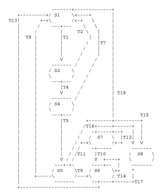
The following state transition table represents the above diagram. Each row represents the starting state for a given transition, which after taking a transition marked in a table cell would end in the state represented by the column of the cell. For example, from state S1, the connection takes the T1 transition to arrive at state S2. The fields marked "-" correspond to undefined transitions.
