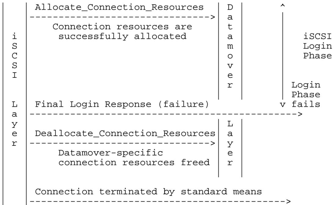
Figure 5 A failed iSCSI login on target
