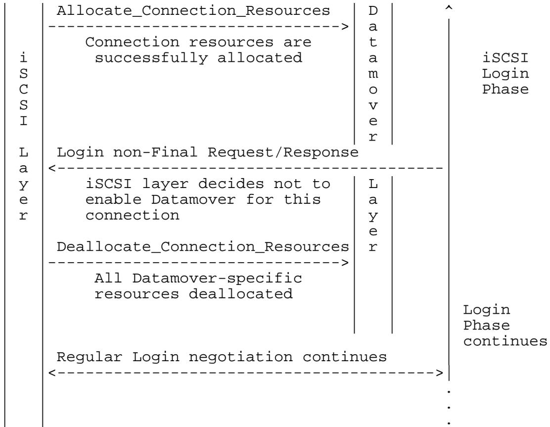
Figure 6 iSCSI does not enable the Datamover
