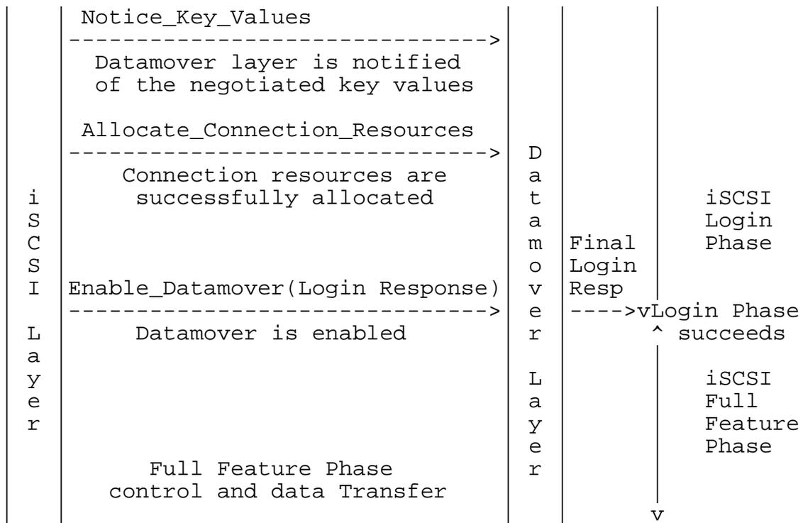
Figure 3 A successful iSCSI login on target
