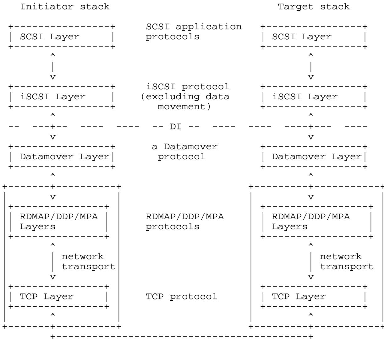
Figure 1 Datamover Architecture diagram, with the RDMAP example
