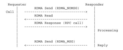
An RPC-over-RDMA transaction using a Long Reply:
