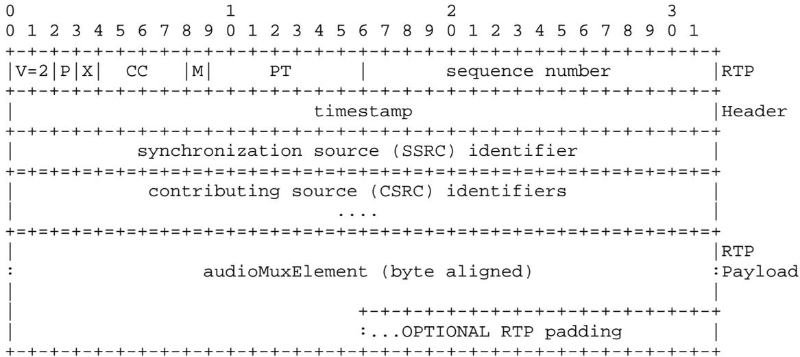
Figure 4 - An RTP packet for MPEG-4 Audio
