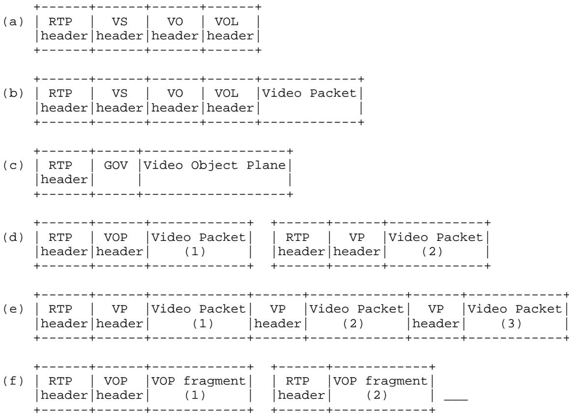
Figure 2 - Examples of RTP packetized MPEG-4 Visual bitstream
