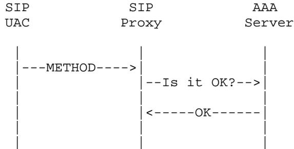
Figure 1: Call flow over the SIP-AAA interface
