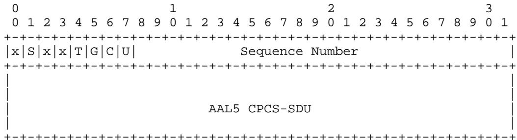
Figure 3: ATM AAL5-SDU Mode Encapsulation
