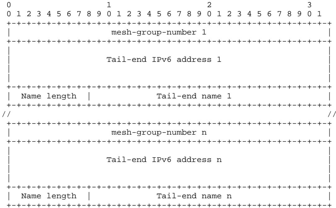
Figure 3 - OSPF TE-MESH-GROUP TLV format (IPv6 Address)
