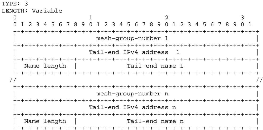
Figure 4 - IS-IS TE-MESH-GROUP sub-TLV format (IPv4 Address)
