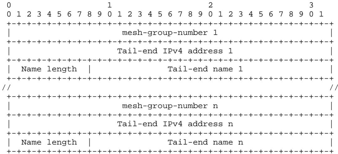
Figure 2 - OSPF TE-MESH-GROUP TLV format (IPv4 Address)
