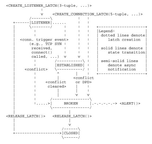
Figure 1: Connection Latching State Machine
