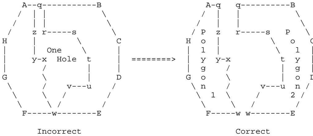
Figure 4: Specification of Hole with Multiple Outer-Boundary Intersections
