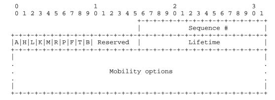
Figure 2: Extensions to Proxy Binding Update Message
