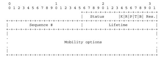
Figure 3: Extensions to Proxy Binding Acknowledgement Message
