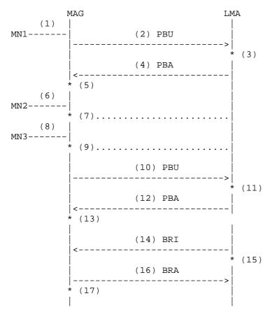
Figure 1: Exchange of Group Identifier
