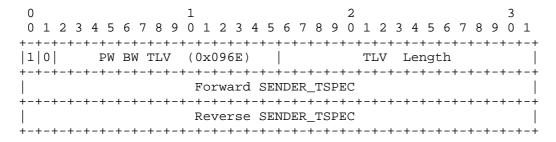
Figure 5: PW Bandwidth TLV Structure
