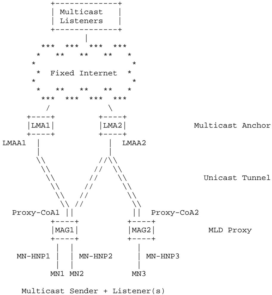
Figure 1: Reference Network for Multicast Deployment in PMIPv6
