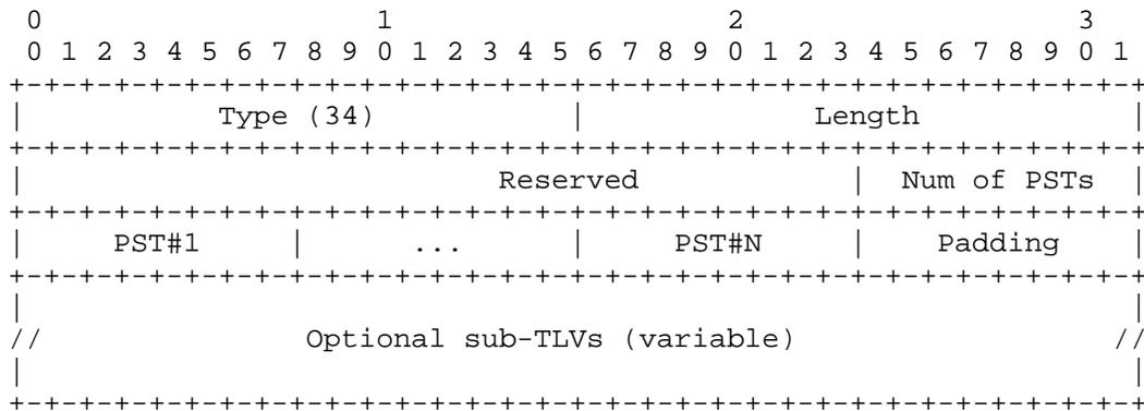
Figure 1: PATH-SETUP-TYPE-CAPABILITY TLV
