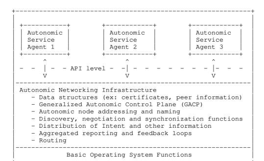
Figure 2: Model of an Autonomic Node
